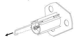
11. If you are using a core, slide it onto the rewind spindle until it is flush against the guide plate.
